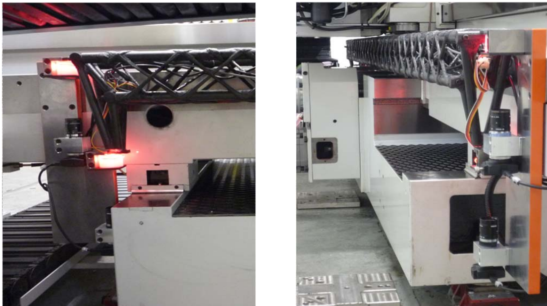
Figure 3-12 – Left and right side camera sensors
