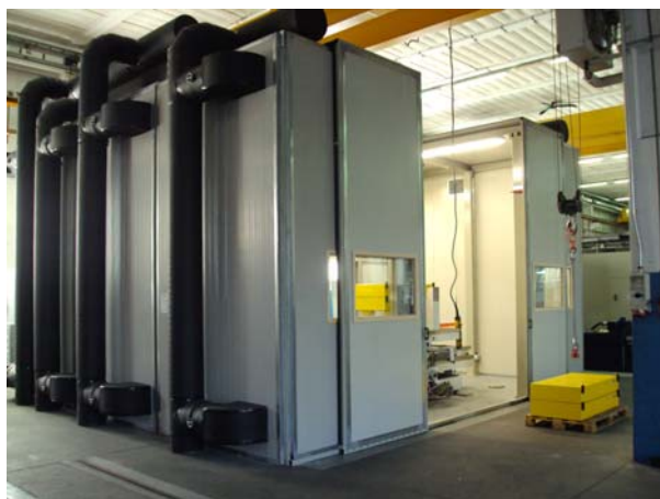
Figure 3.3 – SOMMACT demonstrator test chamber with mass loading-unloading facilities
