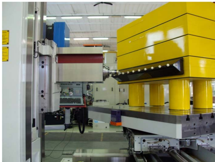
Figure 3.7 – The 3D reference beam directly applied to the demonstrator test masses
