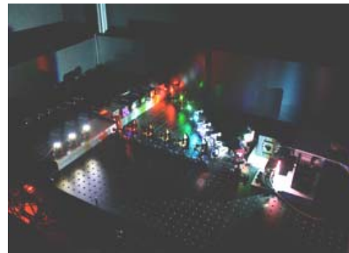
Customized Andor Revolution Spinning Disk Confocal microscope of CiBIT microcopy unit. Upper: Olympus IX81 inverted fluorescence microscope with environmental control box. Lower: Customized laser combiner
