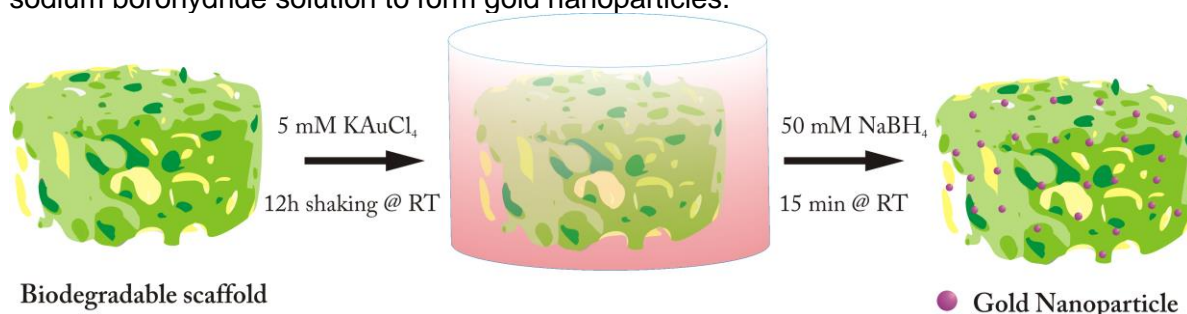
Scheme 3: Schematic representation of the fabrication of the gold nanoparticles decorated scaffold.
