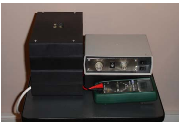
Fig.2 Photo of lab-scale LED-based light source emitting light at 589 nm.
