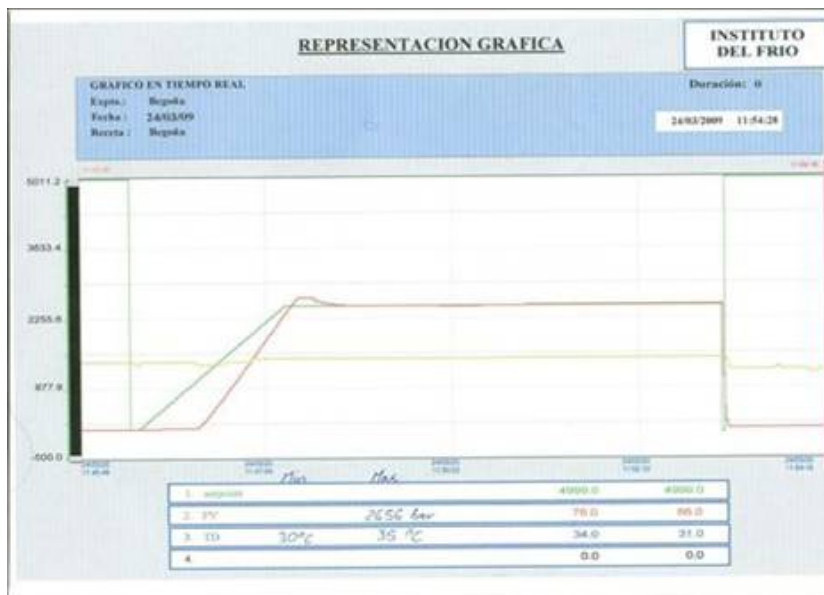
Graphic 1: Graphic of treatment parameter (pressure, temperature, time of treatment) of combined process High Pressure / Temperature recorded in the Instituto del Frío HP equipment during all the phases of the process.
