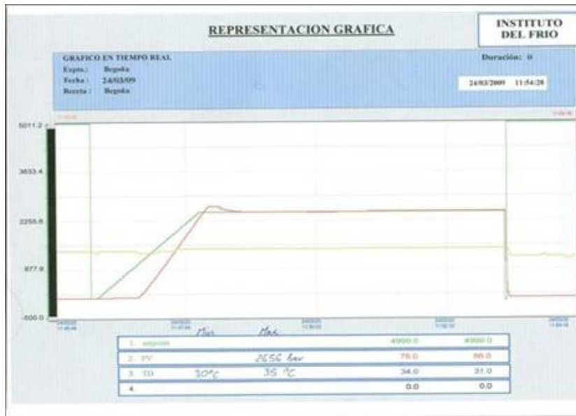
Graphic 1: Graphic of treatment parameter (pressure, temperature, time of treatment) of combined process High Pressure / Temperature recorded in the Instituto del Frío HP equipment during all the phases of the process.
