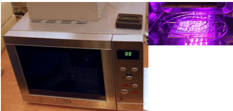
Fig.1 Photo of pilot-scale LED-based light source prototype with LED's matrix emitting light from bottom and from top.
