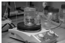
mix and heat vigorously (a magnet's doing the mixing)
