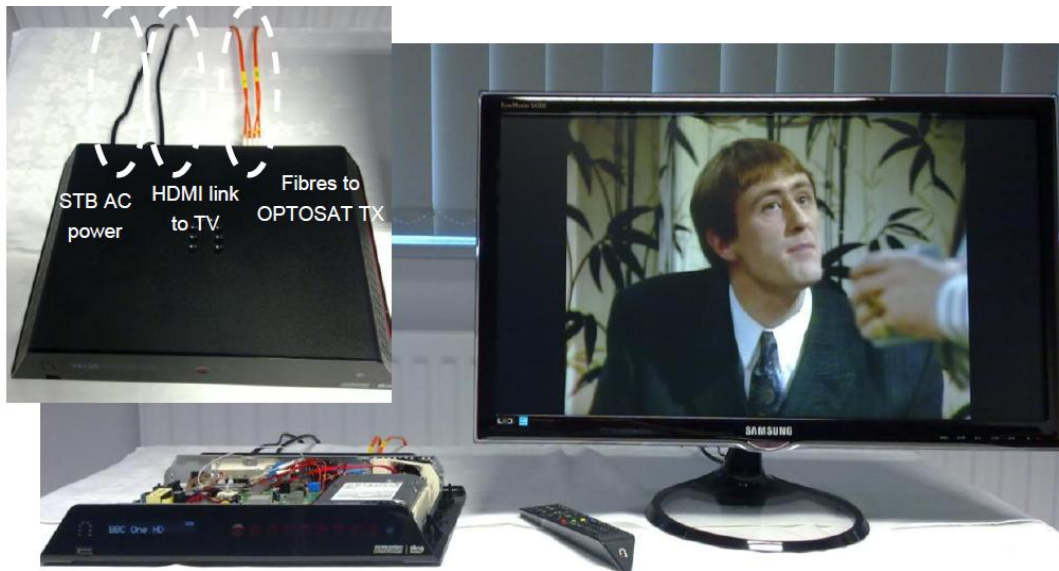
Figure 15 Block diagram and photographs showing the STB with integrated Optosat receiver circuitry, and showing the unit used to display live TV signals
