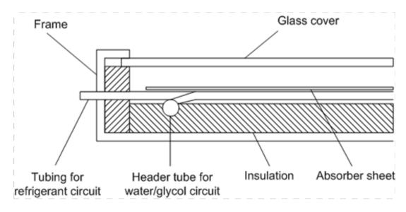
The inclusion of refrigerant pipes in the solar collector allows us to utilise radiant heat energy in the air- source heat pump operating mode for space heating: this will happen when there is space heating demand and the levels of solar radiation are insufficient to bring the solar collector water temperatures up to temperatures higher than the stored water or when the solar collected water temperature has reached it's set point.
