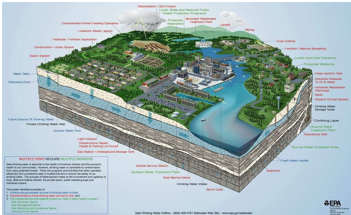
Figure 1: Diagram of the main sources of groundwater contamination (From US Environmental Protection Agency, http://water.epa.gov/action/protect/landscapeposter.cfm )
