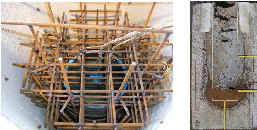
Figure 10: MOCKA 3.1 - View of the rebars before concrete pouring (upside-down) and post-test cut of the test section
