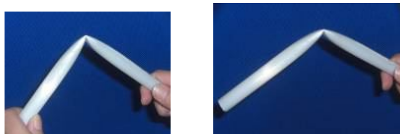
Figure 4. Tube obtained using the new biodegradable compound. Tube aplying strain (left) and tube without aply strain (right).
