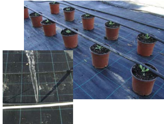
Figure 7. Validation of field of the Bio Pipes. Break in the pipes in the folding line.
