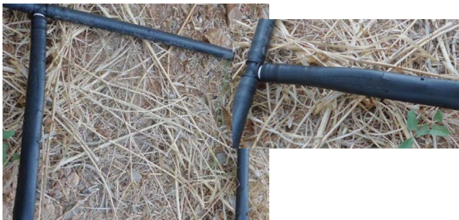
FIGURE. 2. MICRO-IRRIGATION PIPES OBTAINED AT INDUSTRIAL LEVEL PLACED IN-SOIL. DETAIL OF THE WATER INTAKE BY THE DRIP.
