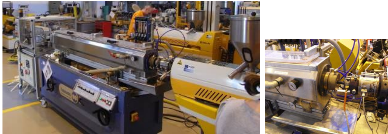
Figure 5. Pilot plant equipment to obtain pipe.
