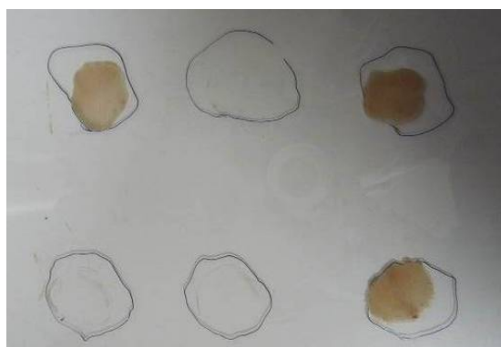
Figure 6. First set of trials: sampling areas before (brown) and after (transparent) sampling with the prototype.
