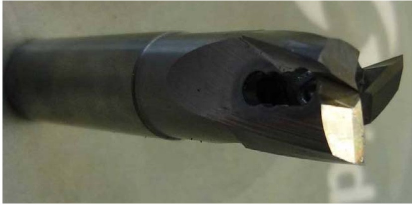
Figure 11. The influence of the cutting edges geometry on the size and shape of the chip and dust has been analysed on this WP4
