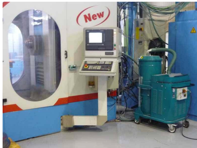
Figure 5 Pilot System including the Aspiration Pump. Aspiration Pump is connected to spindle rear by flexible tube and to machine tool CNC by electric cord
