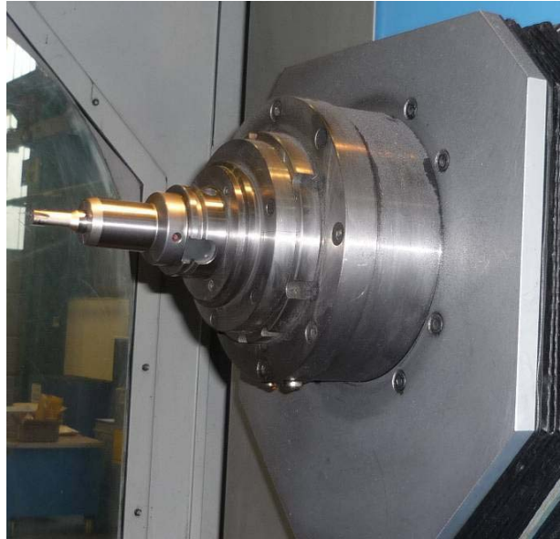
Figure 6 Modified machine spindle with a HSK50-F hydraulic chuck holding a steel tube PCD aspiration tool.
