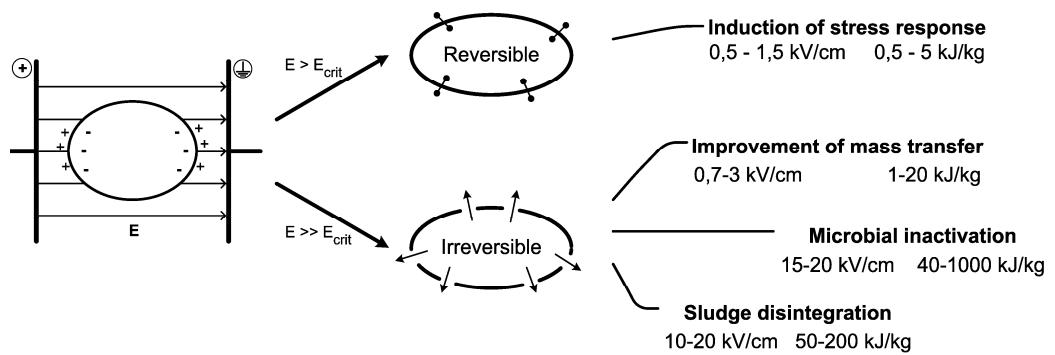
*PEF applications as a function of electric field strength and energy
