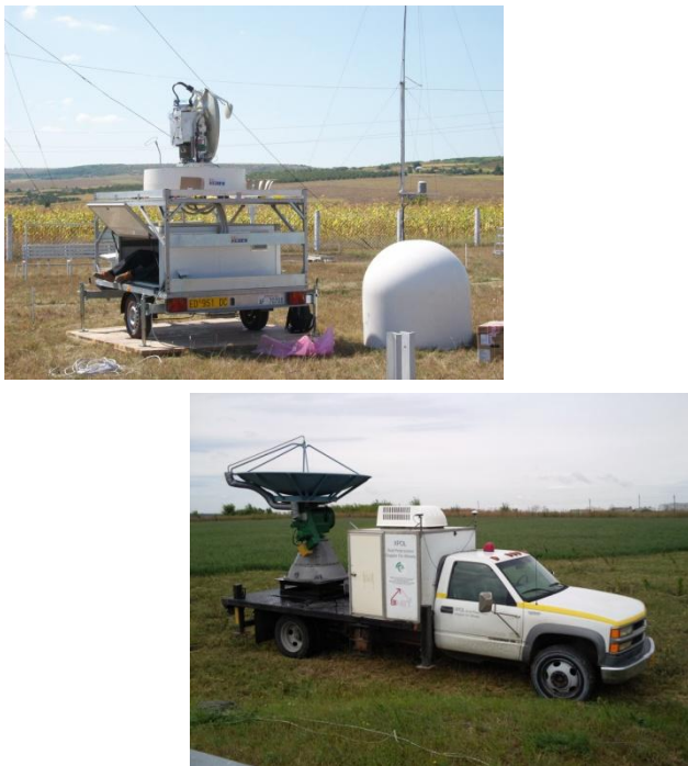
Mobile WR-25XP unit at Baltata site (top) and X-POL benchmark radar at Chisinau (bottom) during the installation phase
