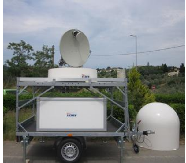
The mobile WR-25XP radar is securely fastened to a trailer that can be easily moved by a car or a small truck
