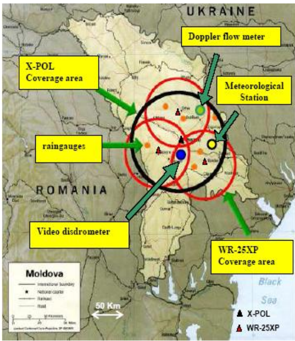
The locations of the available instrumentations for Moldova Operational Field (MOF) campaign. The coverage area of each radar system is also shown
