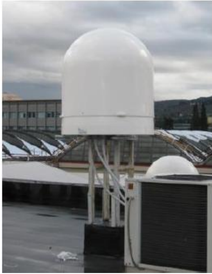
Fixed tower-based WR-25XP radar: transmitter, receiver and antenna parts are inside the radome
