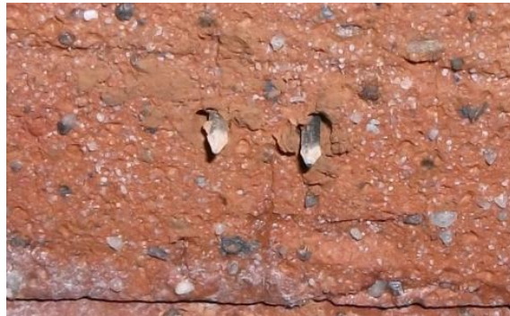
Left: Nails 3-4 in LWC concrete; right: Nails 7-8 in Thermalite
