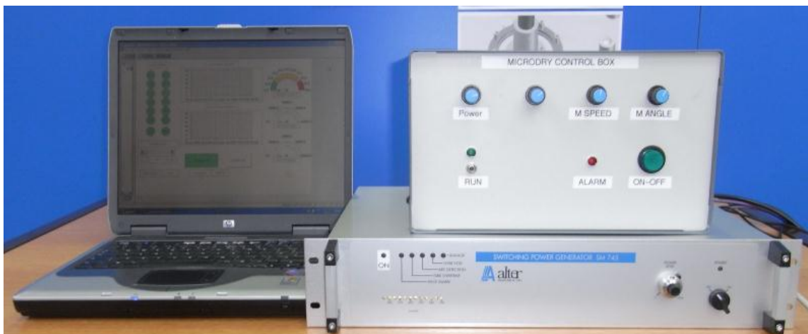
Microwave Power Supply with the PLC Control Box & Computer Interface
