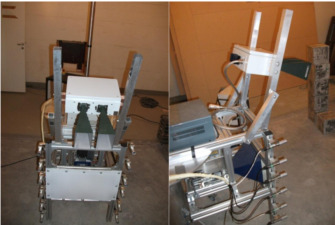
Microwave Moisture Sensor Prototype II mounted on the Microdry unit
