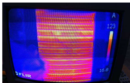
Four prototype ( final prototype) fire test. Tested according to EN 1634-1:2008
