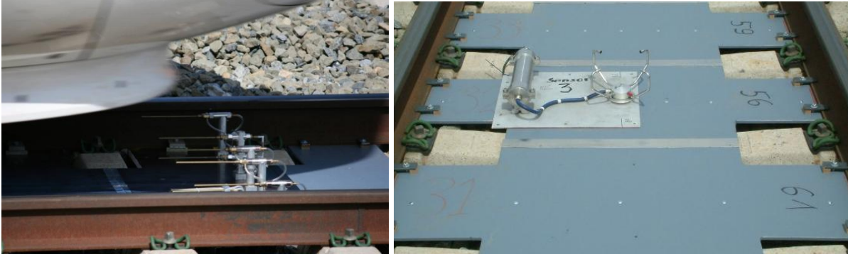
Figure 3: Sensors used to measure the flow patterns under a High Speed train.
