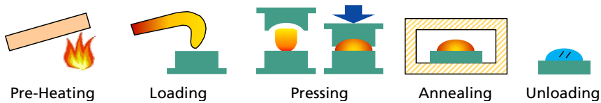
Figure 3-3: EcoGlass moulding concept
