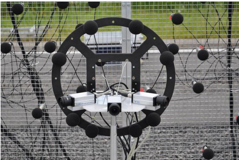
**Figure 14.** Panoramic camera module with three cameras at -60, 0, and 60 degree
