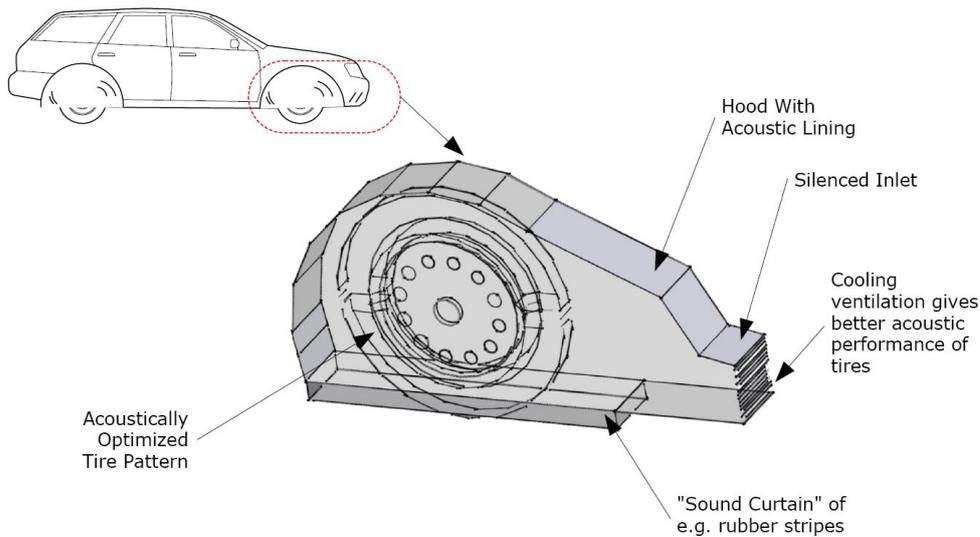
**Figure 8. The concept of tyre hoods for reduction of tyre/road noise. Note: The silenced cooling air intake to keep tyre temperature down. The rubber stripes reduce the air gap to the road surface.**
