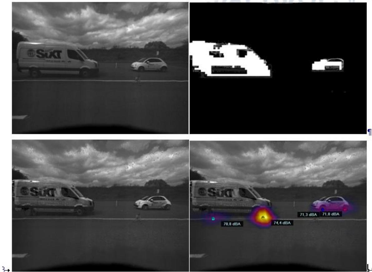
Figure 15. Object detection in real time: original video image showing two vehicles (upper left image), image analysis, foreground segmentation and object identification (upper right image), video morphing (lower left image), beamforming and calculation of source levels (lower right image)
