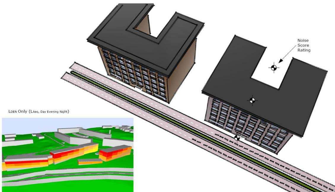
Figure 4. Improved indoor hot-spot analysis. Hot-spot analysis means that indoor and outdoor noise data are weighted together to a total noise score value. More factors will also be considered in the improved noise score model.
