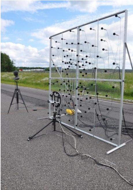
**Figure 13.** Grid structure (3 x 3 m) with 120 microphones in a random pattern
