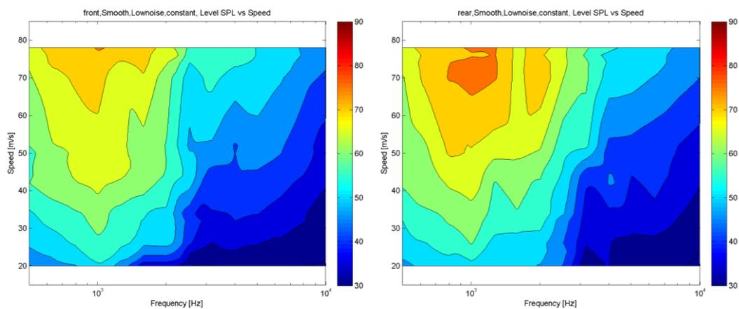
Figure 16. Example of an Acoustical Fingerprint; Left: Front tire, smooth surface, low noise tires, Level [dB(A)] vs. speed and frequency; Right: Rear tire, smooth surface, low noise tires, Level [dB(A)] vs. speed and frequency
