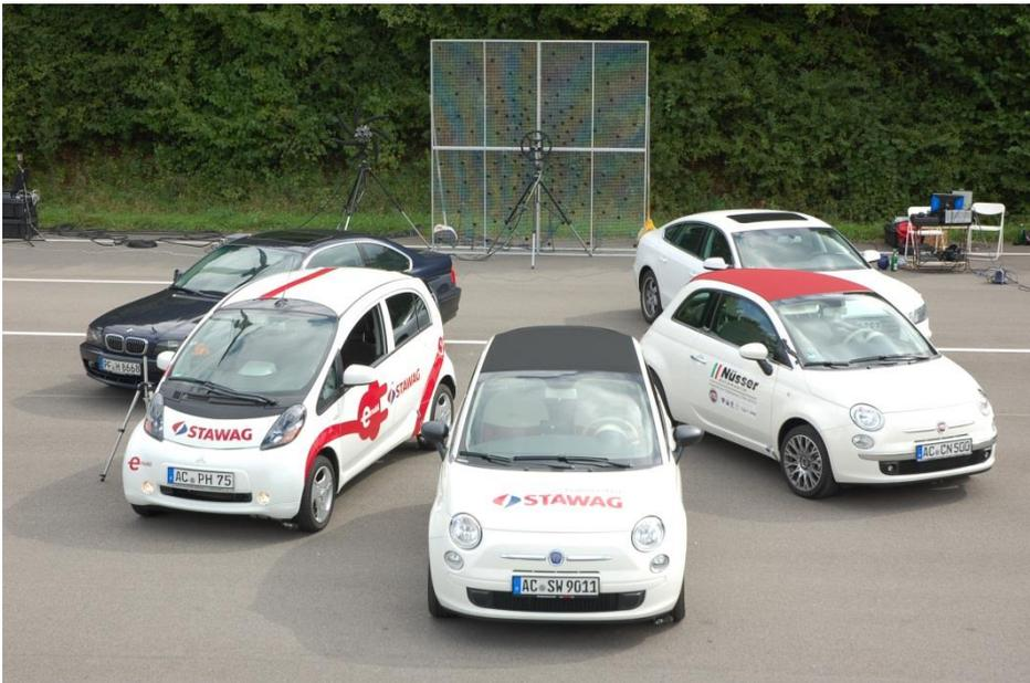
Figure 17. Measurement campaign with 5 different passenger cars (2 electric vehicles, 3 ICE cars) on test track using the developed modified head visor microphone array
