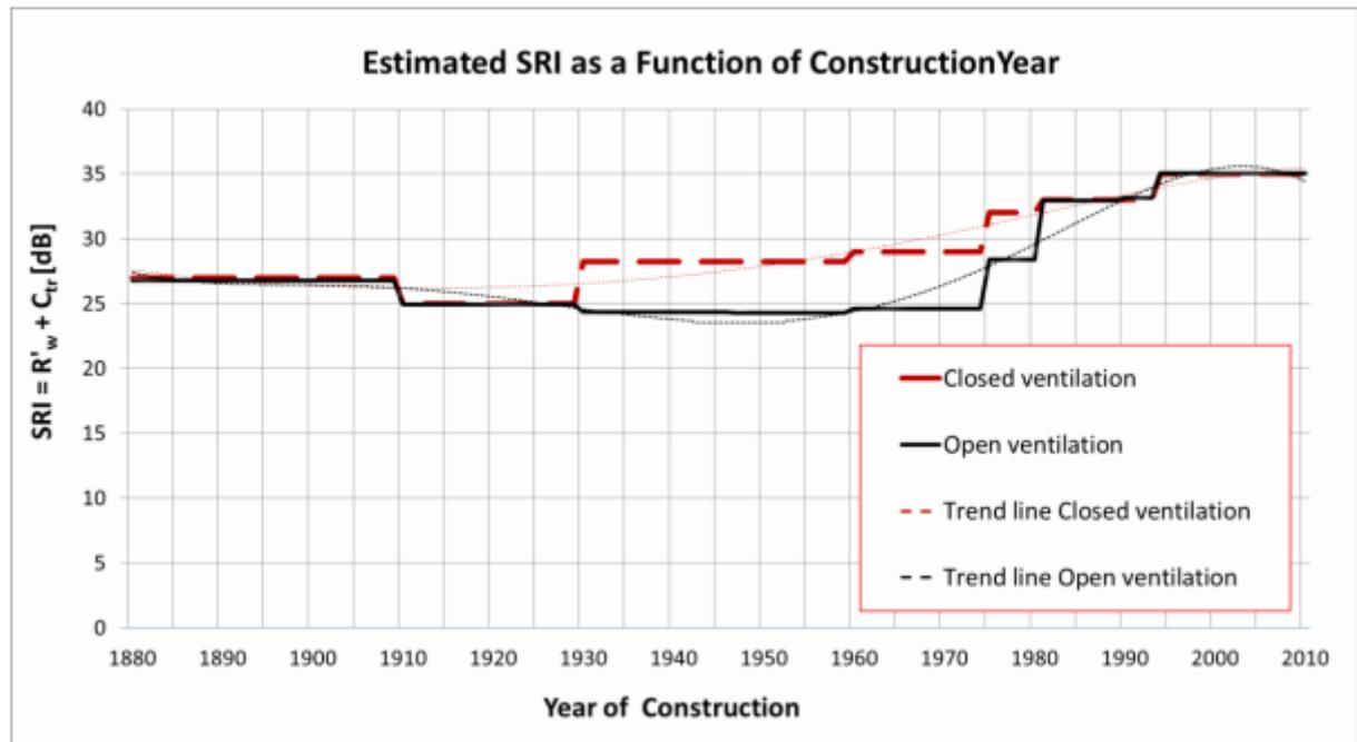
Figure 11. Estimated SRI as a function of construction year for Stockholm test site.
