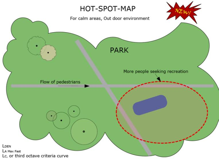
Figure 5. Hot-Spot analysis for the outdoor environment, e.g. in parks. Outdoors, the population density, equivalent and maximum sound levels as well as the low frequency content will be considered in the noise score value
