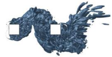
Figure 17: Q iso-surfaces demonstrate the flow topology for the two struts test case
