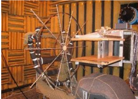
Figure 6: Onera's microphone antenna in ECL's wind tunnel
