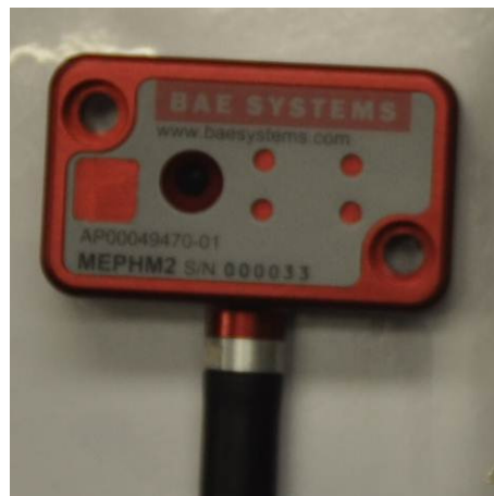
Figure 10 Tiny Micro Electronic Prognostic Health Monitor (MEPHM)
