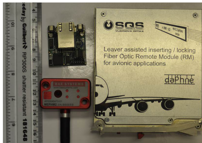
Figure 11 MEPHM and media converter in size comparison to remote module (RM) box
