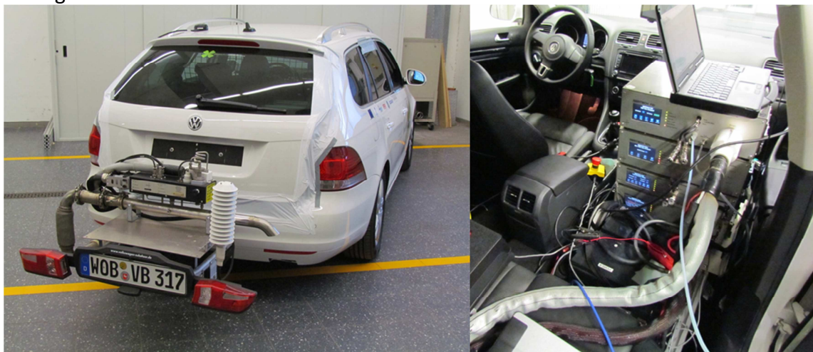
Fig. 2 PEMS installation on the final validator vehicle
