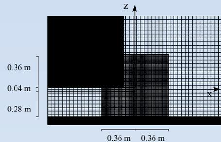
Figure 2. Cross section of Figure 1 at  $y = 0$  discretized with coarse and fine grids according to the multi-domain FPS method.
