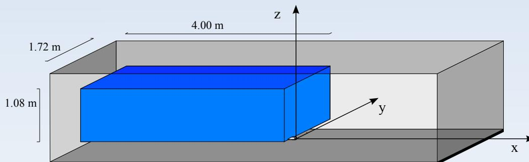
Figure 1. Configuration of an exhaust pipe (orifice located at the origin of the coordinate system) in the presence of a rigid ground surface and simplified automotive body. Computational boundaries are shown.
