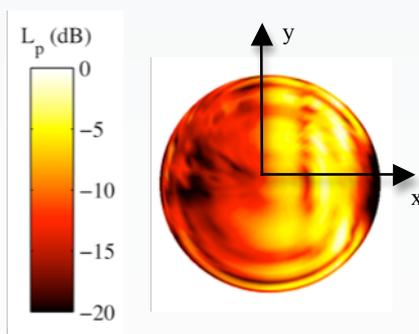
Figure 3. Snapshot of impulsive sound radiated from the tailpipe in the cross section of Figure 1 at  $y = 0$ . a) no jet, b) hot jet.  $L_p$  relative to maximum level.
