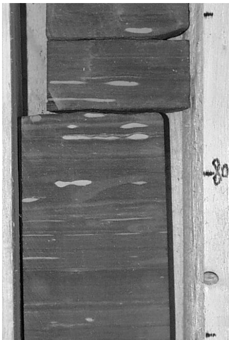
Fig.1: Autochthonous phosphate nodules in silty marl matrix of Schöneck Formation. Site Oberschauersberg 1
