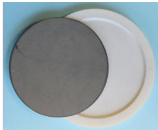
Fig. 4 Cross-section and sintering dies of gravity sintered NiCoCrAlY discs
