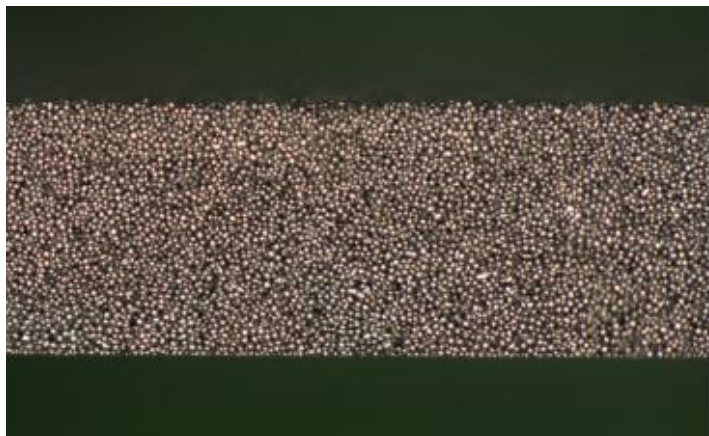
Fig. 4 Cross-section and sintering dies of gravity sintered NiCoCrAlY discs
