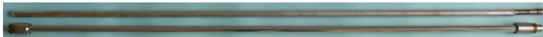
Fig. 2. Picture of 1m long pure Pd membrane tubes equipped with IMR seals (on the top) and ECN seals (on the bottom).
