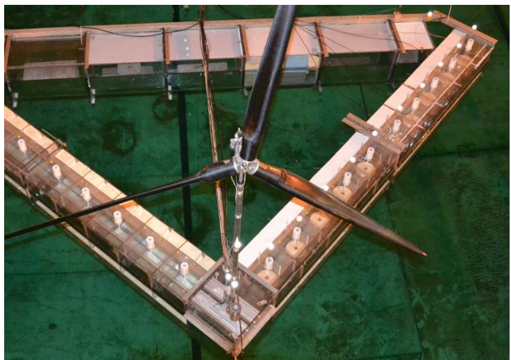
Figure 16: Test models of the SFC (left) and the OWC Array (right) concepts in the ocean basin at ECN
