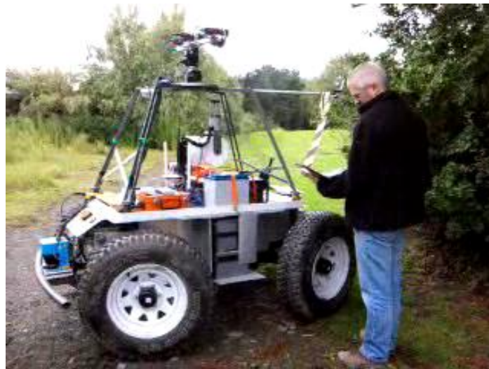
Figure 28: The Idris rover undergoing remote software integration tests outside at the AU Robotics Workshop. Note the heavy-duty PTU has been replaced with the standard AU PTU and only the AUPE-2 cameras were used during Integration Campaign 5.
