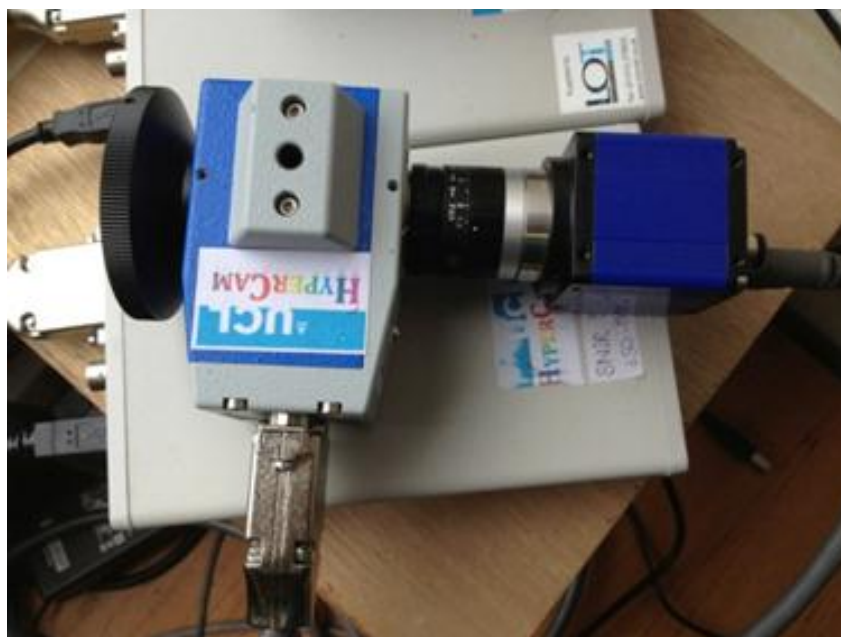
Figure 13: HyperCam optical head composed of Blue Fox CMOS camera, C-mount lens and LCTF (adapter but not stray light baffle shown); on top of SNIR & VIS control electronics boxes.
