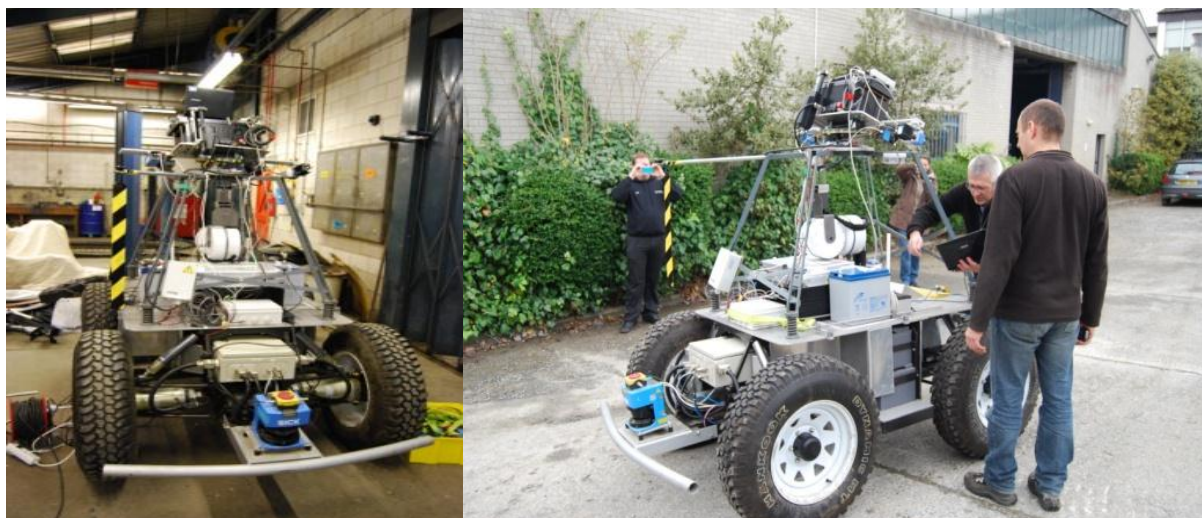
Figure 20: (Left) Sorting out the complex wiring problem when integrating all of the cameras onto the Idris rover platform. (Right) Starting up Idris to begin preliminary integration tests at the AU Robotic Workshop.
