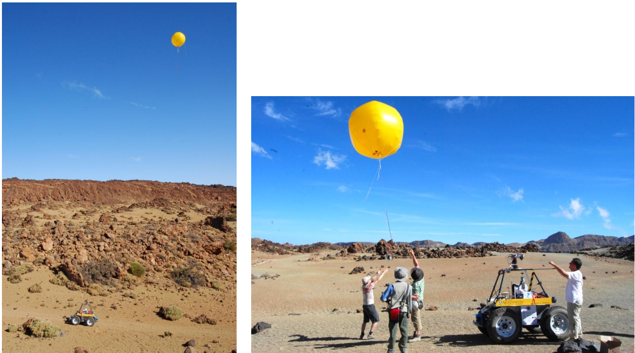
Figure 36: Left: The AU tethered aerobot with aerial camera being towed by the Idris rover during the PProViScout Tenerife Field Trial. Right: A late afternoon flight proved to be problematic given the increased wind speeds and lower atmospheric densities experienced later in the Tenerife day.
