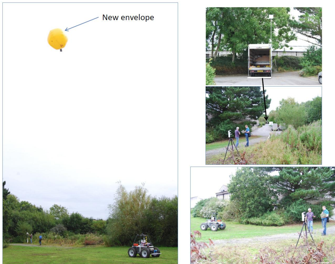
Figure 31: (Left) Testing the new 7' diameter tethered aerobot envelope. (Right) Final tests of the communications infrastructure to assign IP addresses etc. prior to departure to Tenerife. (Right Top) the van with communications antenna was parked some distance away from Idris. (Right Middle/Bottom), the local antenna placed in closer proximity to Idris.
