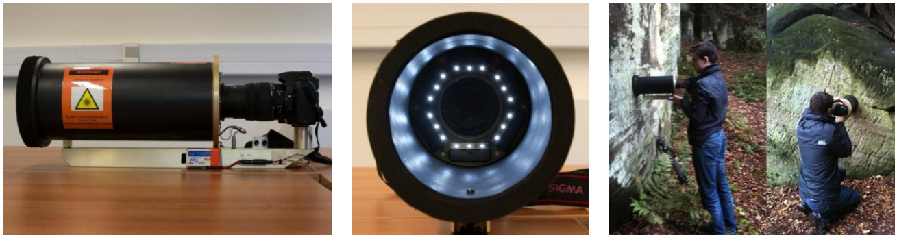
Figure 12: Side view (left) and “Down the barrel” view (middle) of the second version of WALI showing the white LEDs. The light-tight barrel obviates the need for a blackout tent. Right: Field testing of WALI 2 on photosynthetically-colonised rock surfaces in Tunbridge Wells.
