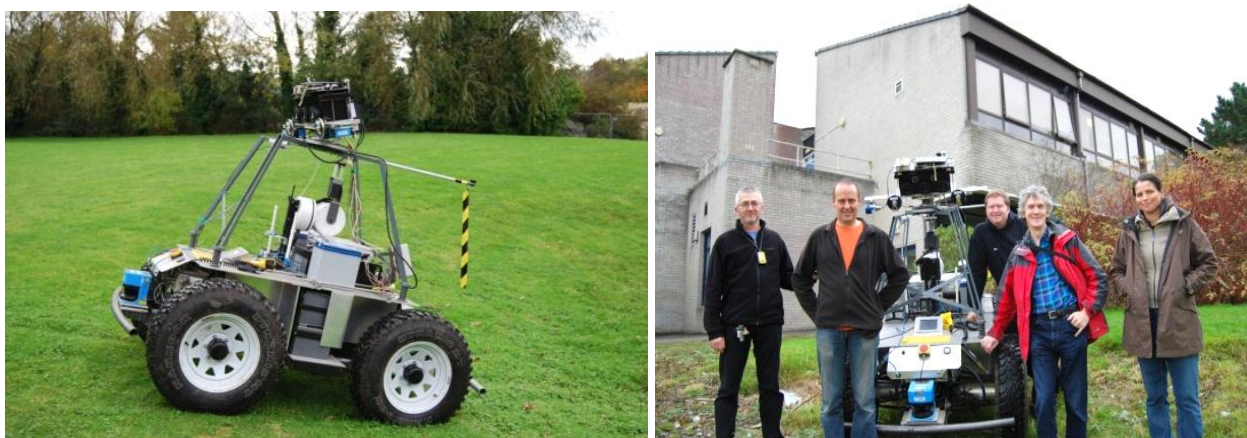
Figure 21: (Left) "Shake-up" of the Idris rover with mounted cameras to test the mechanical integration. (Right) Members from the CSEM and AU partners during the Integration Campaign 3 at Aberystwyth.
