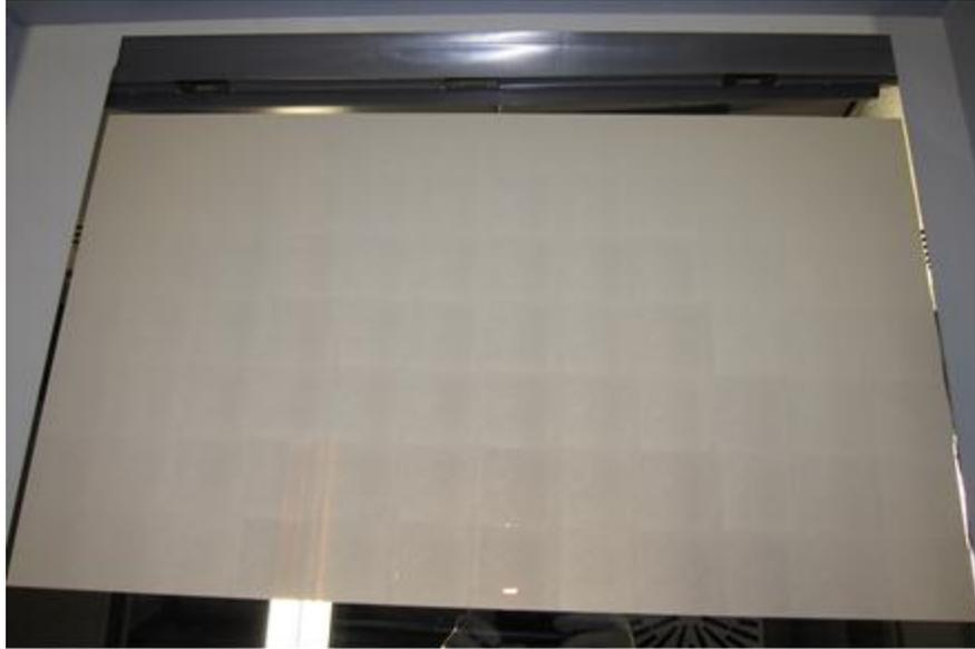
Figure 3: Large area (30x60 cm<sup>2</sup>) nickel master (father) with random ZnO Z5 texture after electroforming
