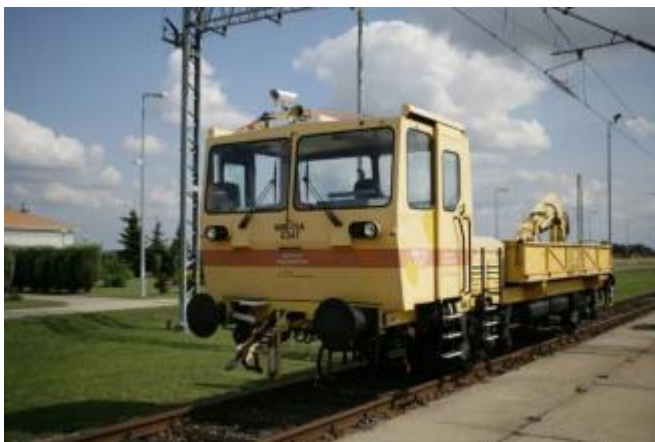
Figure 54 Camera mounted on the roof of the tractor (left) and sample image of the Change Detection system used for railway monitoring (right).
