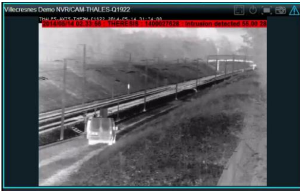
Figure 62 Intrusion Detection at night time (thermal camera)
