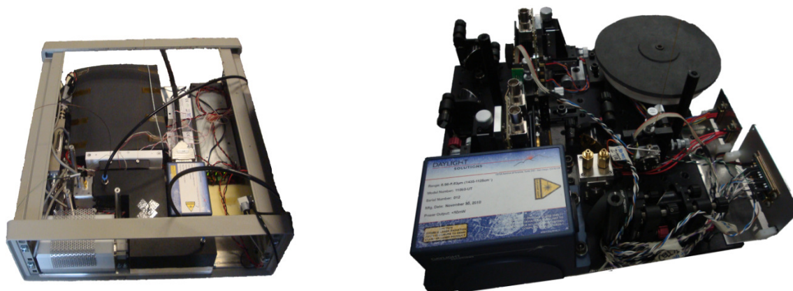
Fig. 17: HF-IRAS analyzers. Left: FRAUNHOFER IPM module, used in the Vapour Detection Unit; right: CREO module, used in the Identification Unit.
