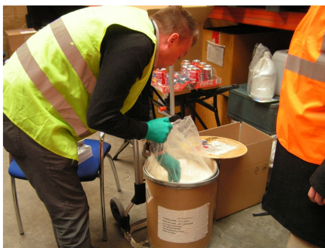
Fig. 31: APAAN smuggled in a cardboard drum. The white powder is packed into two plastic bags (one inside the other). Particles are swabbed from the external bag.
