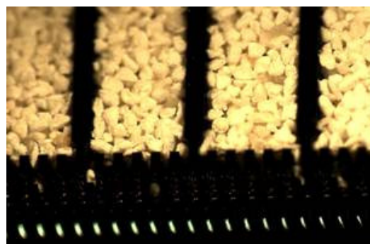
Fig. 14: CNR-IMM Pre-concentration cartridge. Left: the chip. Right: the column packed with a QxCav mesh (by INSTM).
