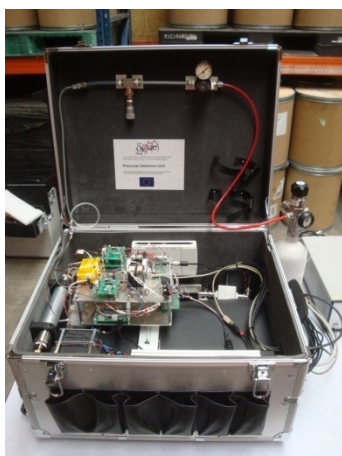
Fig. 3: Vapour Detection Unit. Left: the prototype in its aluminum hand-case. Right: sensing architecture.
