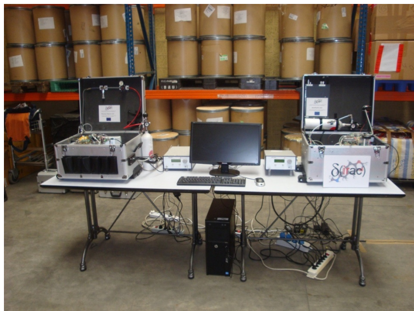
Fig. 30: DIRAC prototypes prepared for the final demo. Vapour Detection Unit on the left, Identification Unit on the right.
