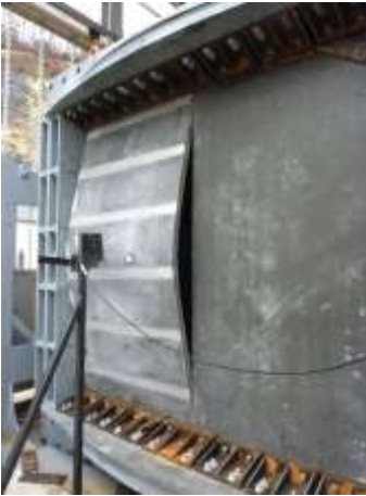
Figure 10 DUCON after shock tube test.
