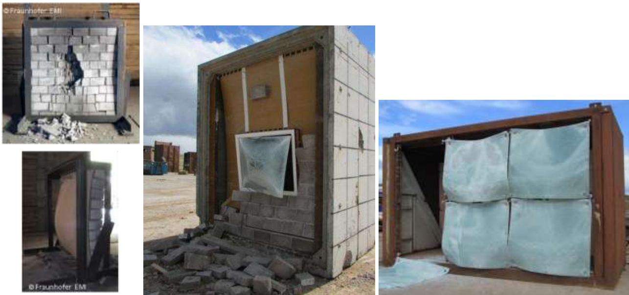
Figure 11 Excerpt of conducted tests: close-in trials with Tecdur® BlastWall (left), free field test with secondary glazing within Tecdur® BlastWall system (middle), point-fixed glazing (right).
