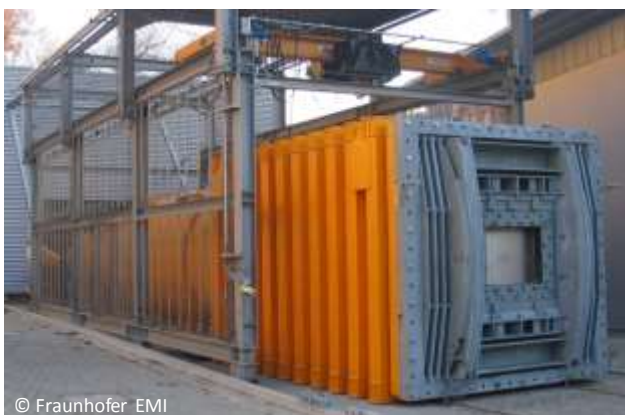
Figure 7 EMI shock tube facility BlastSTAR.
