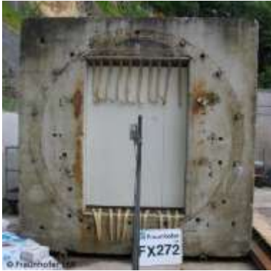
Figure 8 Test set-up of internal detonation test at EMI (left) and at GL Spadeadam (right).
