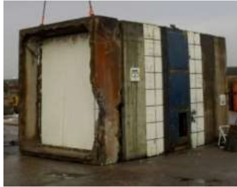
Figure 8 Test set-up of internal detonation test at EMI (left) and at GL Spadeadam (right).
