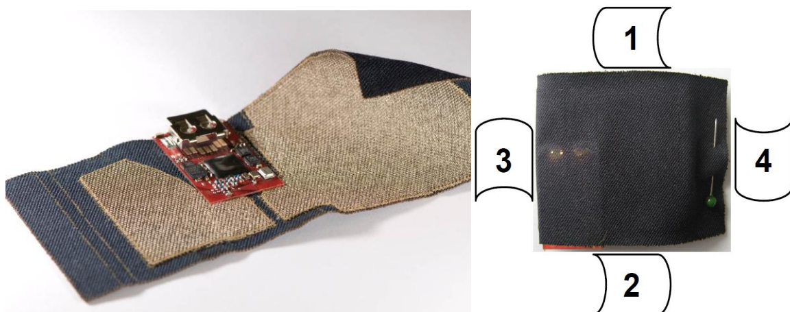
Figure 15: Textile, bendable and lightweight UHF antenna attached to the module
