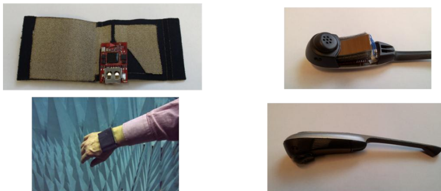
Figure 7: Textile antenna including the Wear-a-BAN electronics, open (upper left), closed on test subject's wrist (lower left), and the headset node antenna (right)
