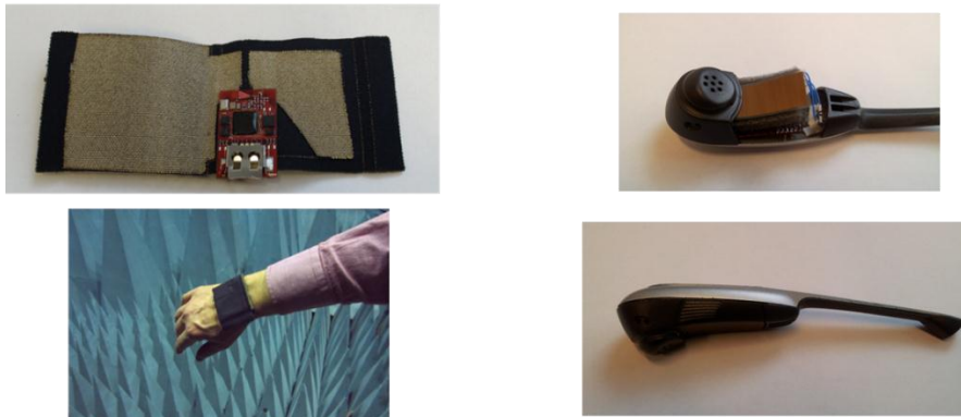
Figure 1: Textile antenna including the Wear-a-BAN electronics, open (upper left), closed on test subject's wrist (lower left) and the headset node antenna (right)
