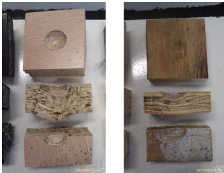
Figure 4: Image of wood samples subjected to drop weight impact test.
