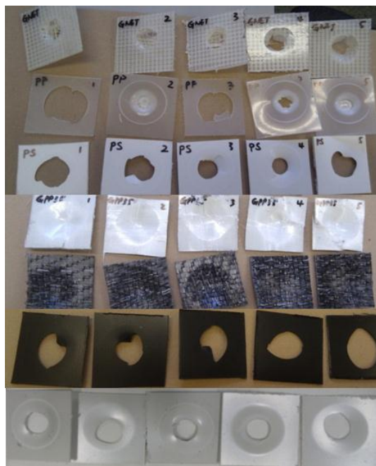
Figure 2: Images of skin samples subjected to drop weight impact tests.
