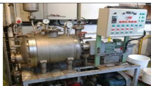
Figure 31: Reactor to carry out enzyme treatment
