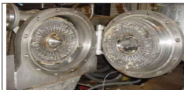
Figure 30: Pressurised refiner to destructure the eucalyptus wood
