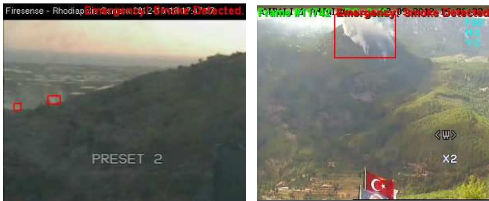
Figure 30: Detection of real wildfires at the archaeological site of Rhodiapolis on 18/10/2012 (left) and near the ancient town of Olympos (Cirali) on 02/09/2012 (right) by FIRESENSE cameras.
