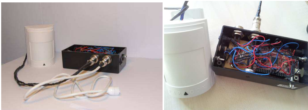
Figure 11: Standalone PIR system. A flood detection sensor is also integrated in the board (the PIR sensor is the white box; the flood sensor is the one with the white cable)
