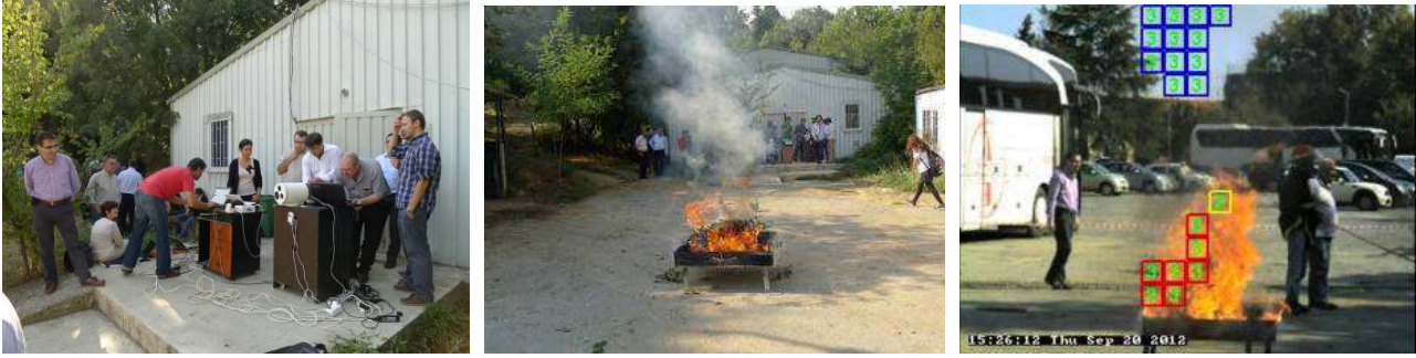
Figure 27: Real fire test in the parking lot of Bogazici University.
