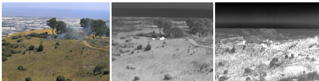
Figure 9: Images from field tests performed in Antalya, Turkey in May 2011 using the Meerkat Fusion multispectral camera: a) visible image, b) SWIR image and c) LWIR image of the same scene.
