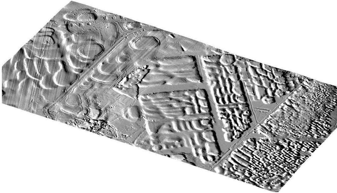
Surface disturbances and subsidence due to underground coal exploitation using chamber and pillar methods, Mpumalanga coal field, South Africa.
