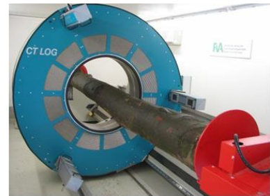
Figure1. CT-scanning of a log.
