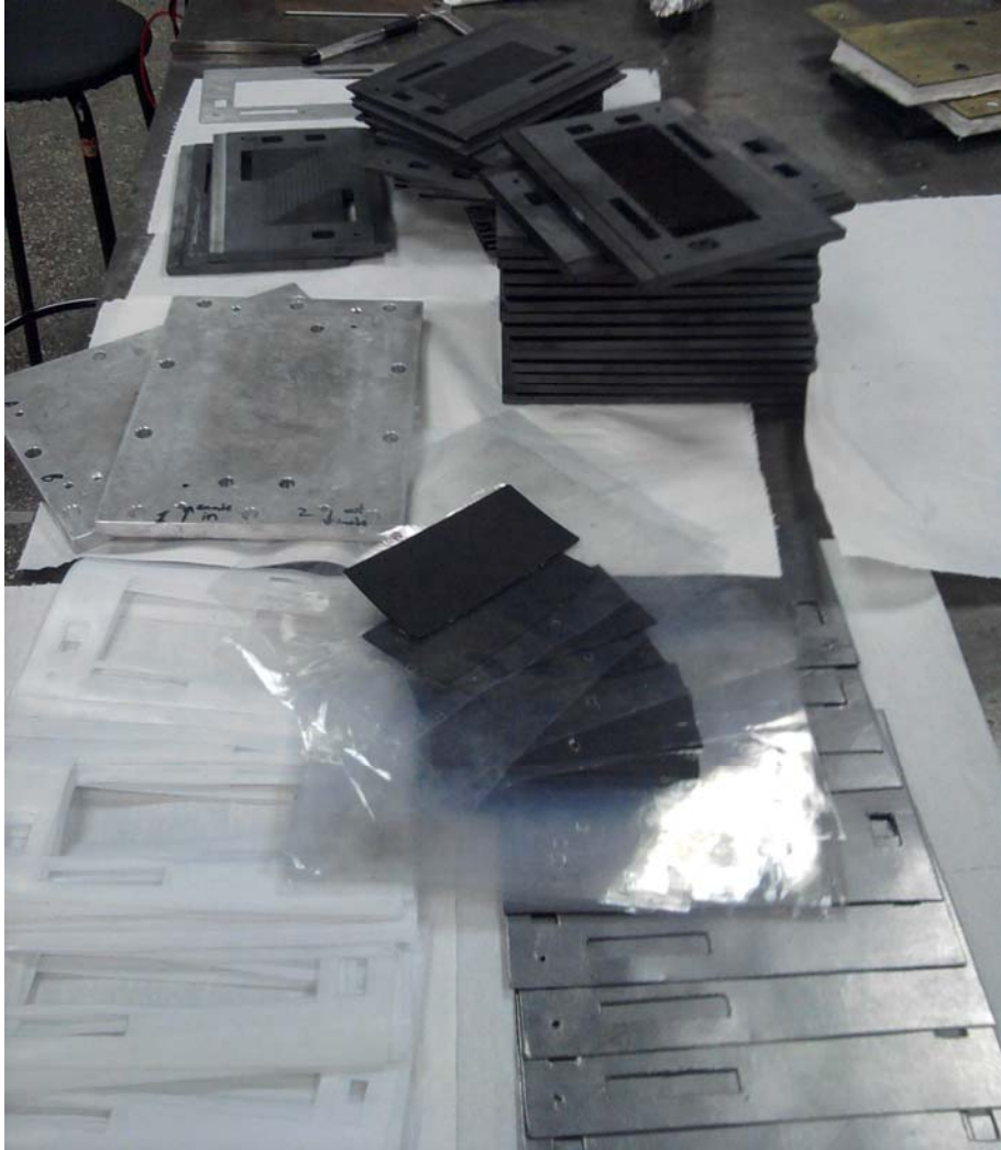
Figure 15: Main components of the final stack (15 MEAs plus 15 reformers; indirect configuration)
