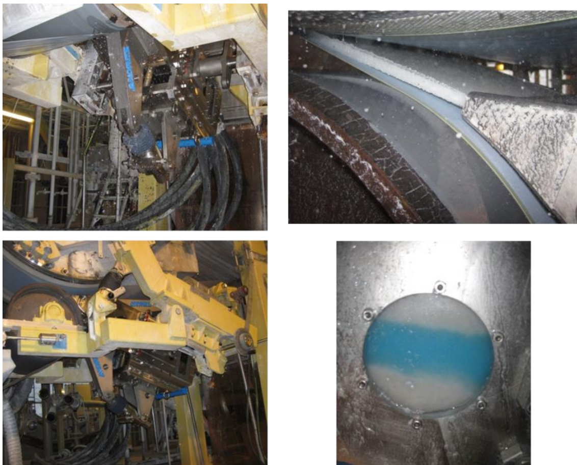
Figure 4. The stratified headbox developed by Andritz, mounted in the FEX pilot paper machine (left, top and bottom). To the right (top) a three layered jet can be seen entering into the paper gap former. Finally at the inspection window mounted in the contraction of the headbox nozzle shows a clearly three-layered structure during the layering demonstration trials.
