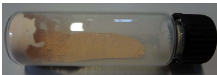
Fig. 9 TTU's catalyst in powder form: 2wt% Pd/MN100 (Source: IMM).
