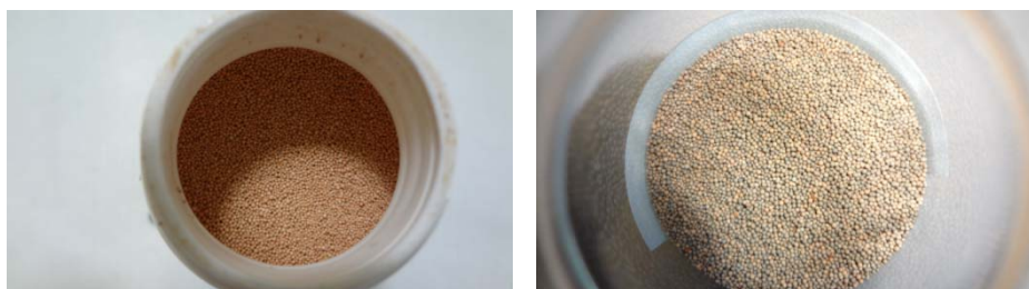
Fig. 8 Left: TTU's catalyst in granular form before; right: after applying in SARD7 reaction (Source: IMM).
