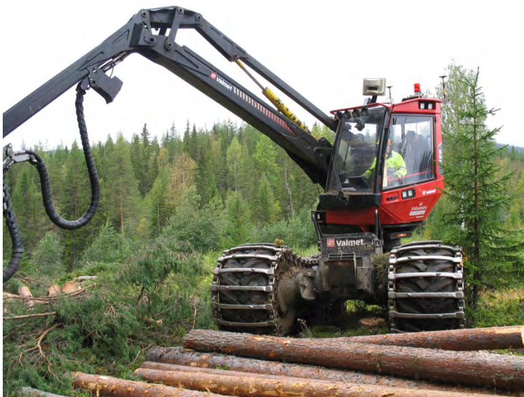
Figure 18. A sensory system for detecting and classifying trees was mounted the cabin of a Valmet 931 harvester from Sveaskog. Photo: Ola Lindroos.
