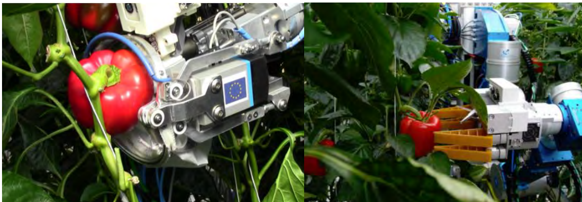
Figure 12. CROPS robot manipulator with the different end effectors in a sweet-pepper crop
