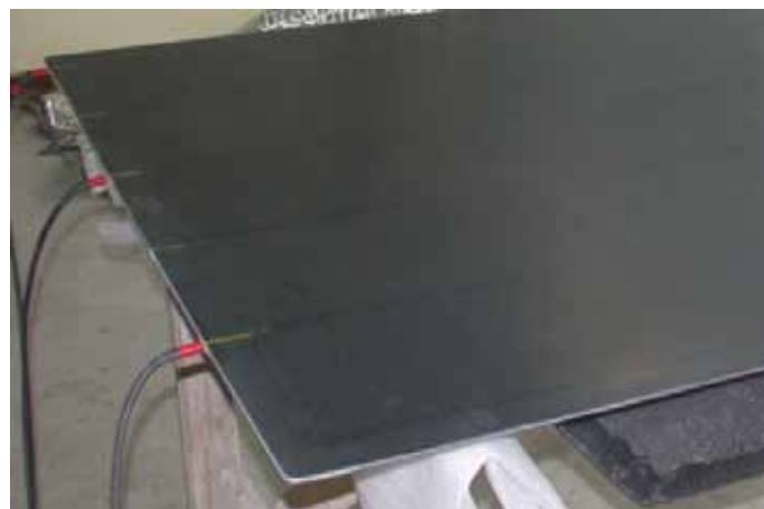
Figure 13 - Fibretemp mould. Detail of the power connection
