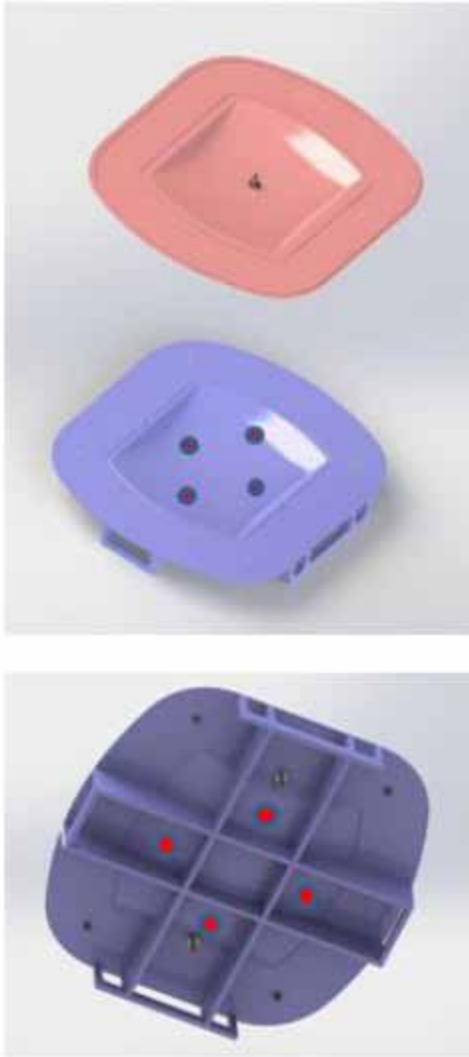
Figure 70- Positions of flow sensors
