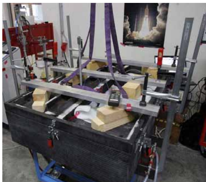
Figure 118 – Tool during injection
