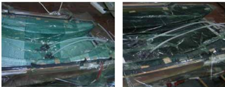
Figure 117 – Infusion process of the second manufacturing step at different time instants (Infusion at 80°C)
