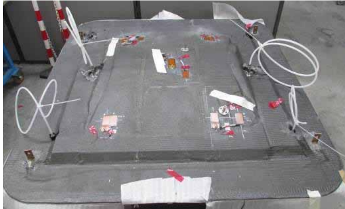
Figure 88 – Lower moulds' rear with an overview of the piezoelectric patches bond to the surface
