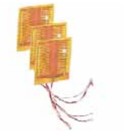
Figure 36- Heat Flux Sensor
