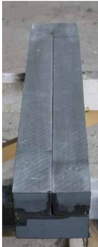
Figure 113 – Complete pultrusion tool (postformer)
