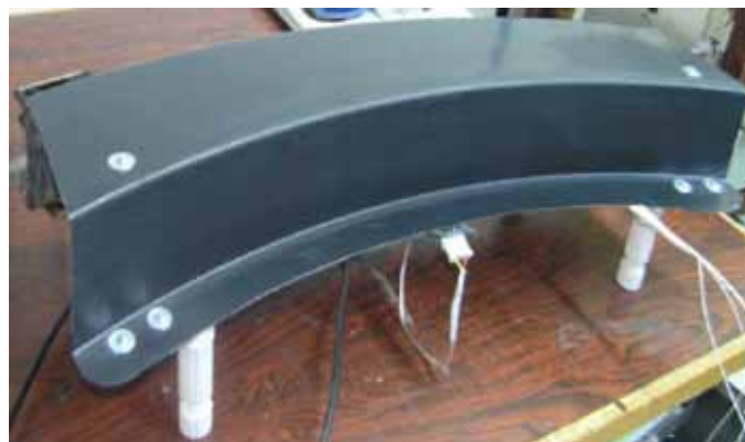
Figure 115 – Self heated infusion tool with gel coat
