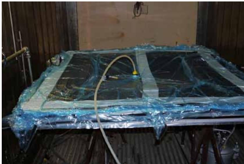
Figure 74: Infusion process to create the heated mould
