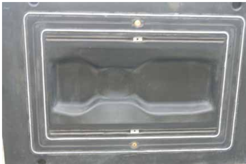
Figure 110 – Finished RTM mould
