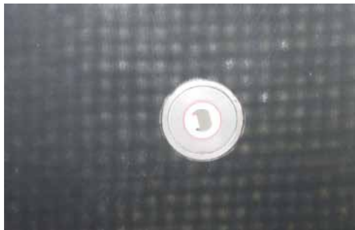
Figure 112 – Integrated dielectric sensor
