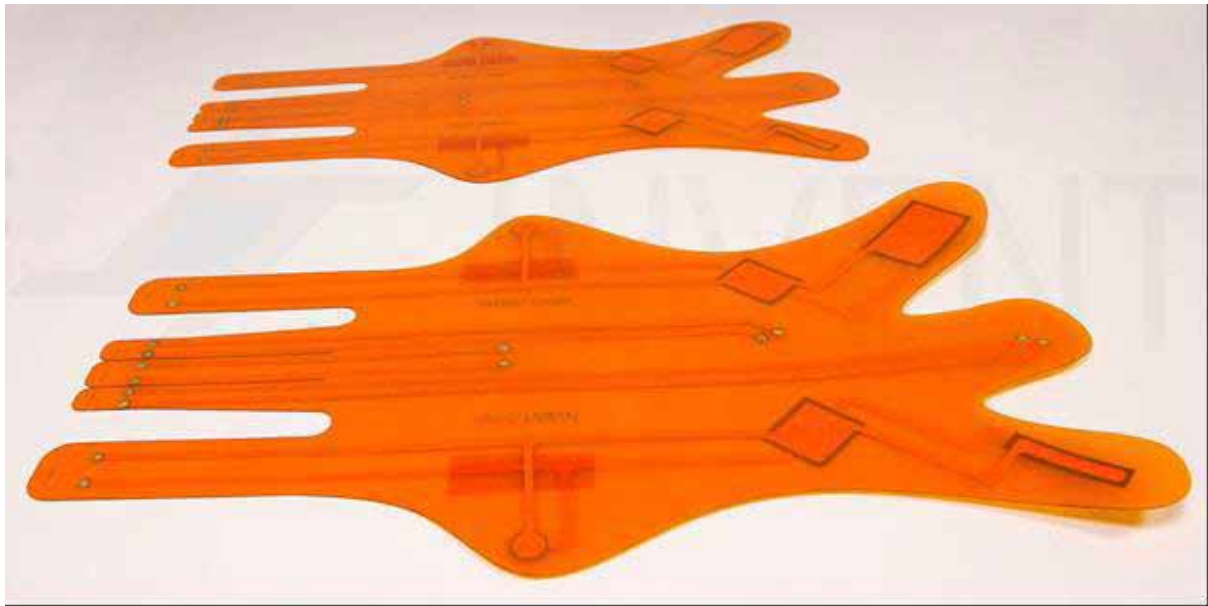
Figure 8 - Prototype of a piezo-electric patch actuator with 6 ceramics, integrated wiring and electrical terminals (Ref: INVENT GmbH).
