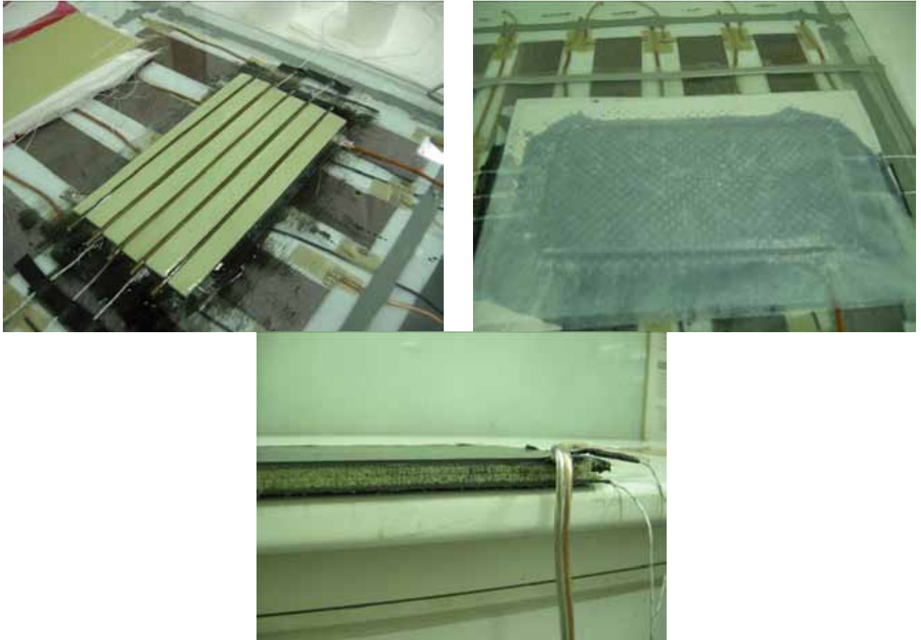
Figure 73. Manufacturing steps of the sandwich structured flat mold
