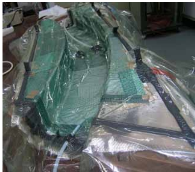
Figure 116 – Manufacturing of the heating element
