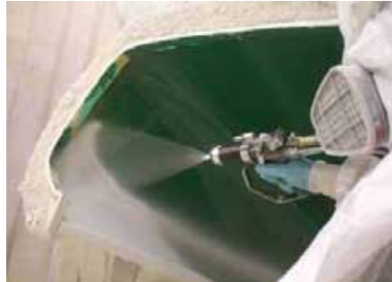
Figure 11 - Example of Gel coat application
