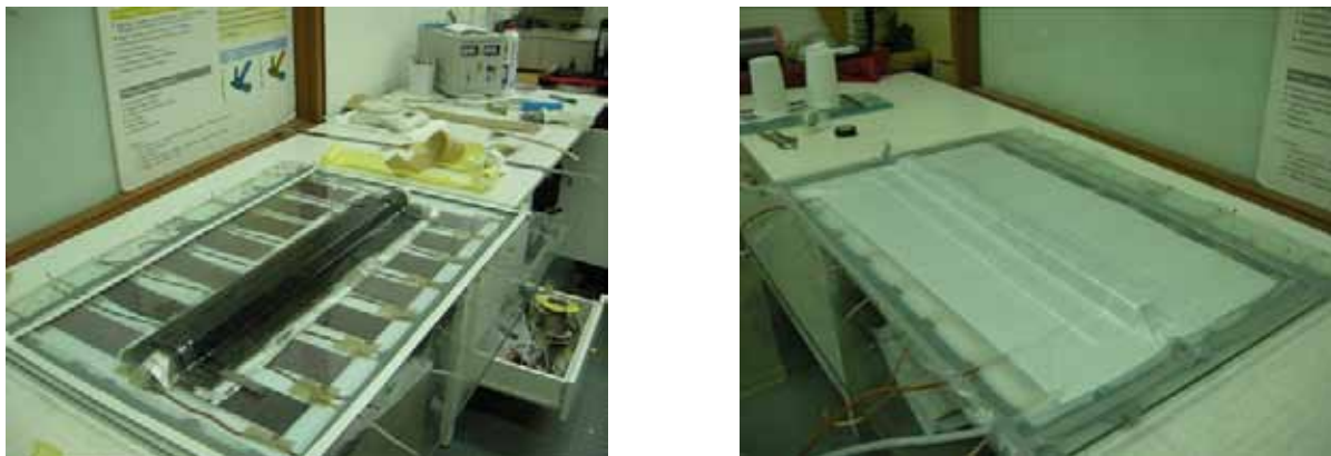
Figure 72. Manufacturing steps of the heating element of the hat-type mold
