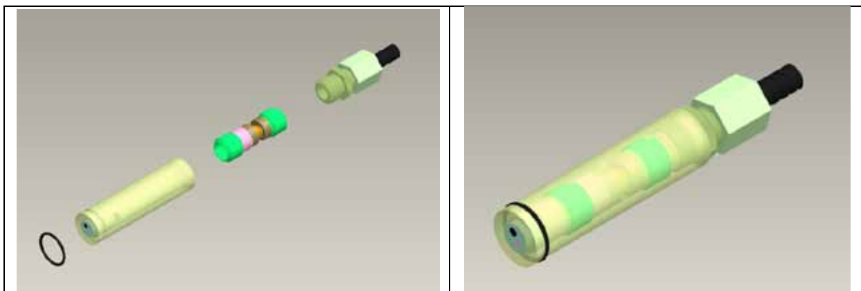
Figure 30 – Flow Sensor – Design details
