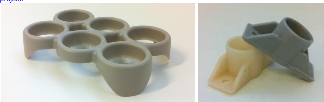
Figure 7. Egg-box and microphone holder produced in the project with different PHB formulations.
