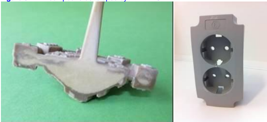
Figure 6. Complex co-injected part (spinning top) and complex injected part (socket) produced in the project.
