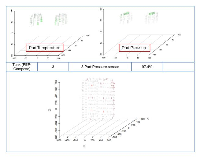
Depending of the case, it is possible to predict the position of 2 to 4 sensors (pressure and/or temperature) to reach 91% to 100% of theoretical prediction of geometrical quality of the parts By working on more sophisticated feature selection methods and classification algorithm, we managed to build a consistent methodology. The methodology is totally new and continued effort is required to make methodology more robust.
