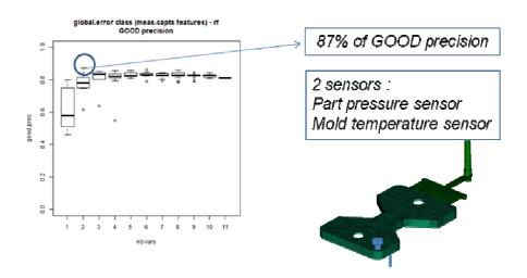
The results on good precision reaches 87% with 2 sensors: a part pressure sensor and a mold temperature sensor. Previously, with the largest nodes selection, good precision attained 93,7%. Here, precision is less high because there are less possibilities of location. Nevertheless, results are acceptable with less computation time.
