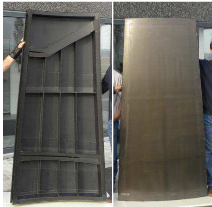
Figure 12: SQRTM Landing Gear Door developed by SCLA and Coexpair
