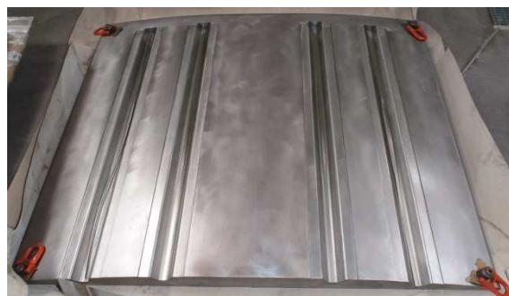
Figure 7 : mould to produce a self-stiffened panel.
