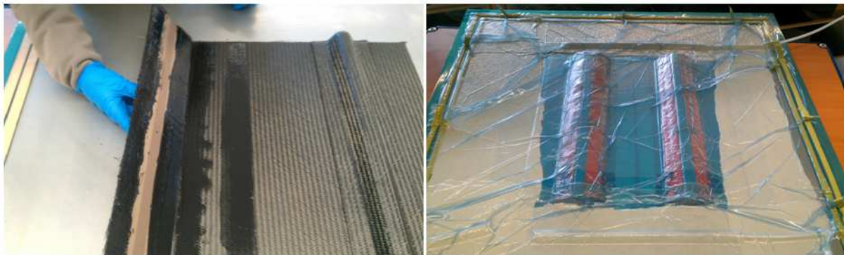
Figure 4: Preform assembly and final bagged part
