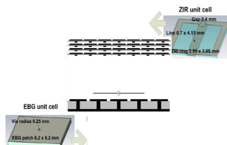
Using EBG and NZ effect to improve gain and directivity of conventional dipole patch antenna
