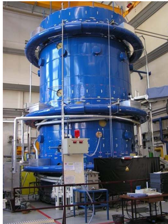
Figure 3: Schematics of the MISTRA facility [3]. Facility characteristics: Main injection lines (lower centered (1), lower off centered (2), upper off centered (3) for steam and incondensable gas) Volume = 99.5\text{m}^3 , Diameter = 3.8m, Height = 7.4m, Compartmented volume.
