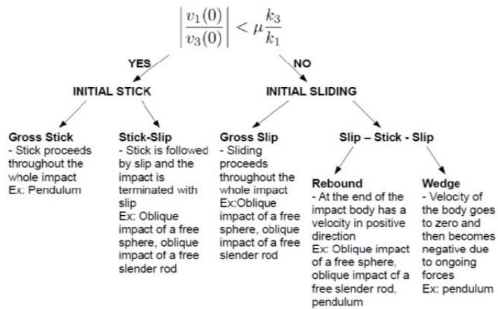
The results produced conditions to avoid wedging (lock-in) so that friction can be related to lift easily. The basic design criterion can be summarized in terms of a critical angle that can be calculated for a given pendulum system.
