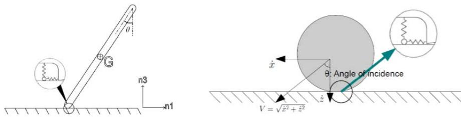
The results produced conditions to avoid wedging (lock-in) so that friction can be related to lift easily. The basic design criterion can be summarized in terms of a critical angle that can be calculated for a given pendulum system.
