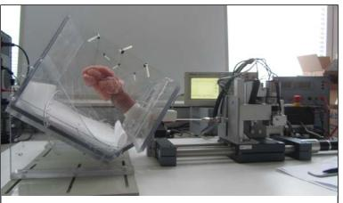
Fig. 2: Testing of the integrated surgical applicator and needle placement robot platform in ex-vivo tissue experiment.
